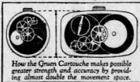
How the Gruen Cartouche makes possible greater strength and accuracy by providing almost double the movement space.
