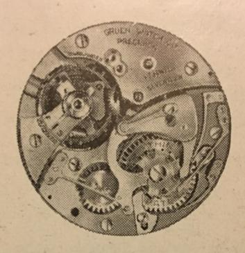
No. 450—"Chrono-timer"—This new and most simple designed movement is called the friction chronograph. This model has a new method of stem fixation, eliminating the detent screw. It has the advantage over the other chronographs in that it is not as complicated, and therefore very easy to be serviced. Has 17 friction set ruby jewels, metalinvar hairspring and monometallic balance wheel. All parts are interchangeable.
