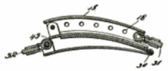
1. In an extension device for a wrist watch rality of sections hinged together to fold on one of said sections comprising two parts sl the other, means for retaining said sections i tion and at the same time preventing sliding one on the other whereby said sections must be slide the parts one on the other.
