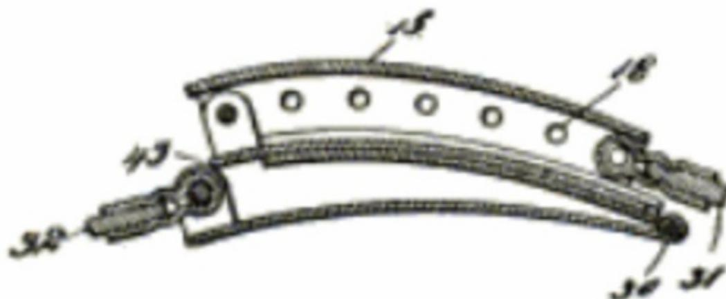
1. In an extension device for a wrist watch, a plurality of sections hinged together to fold one on one of said sections comprising two parts sliding on the other, means for retaining said sections in position and at the same time preventing sliding one on the other whereby said sections must be slide the parts one on the other.
