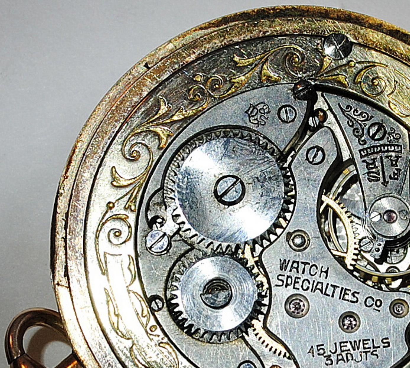
A close-up view of the intricate mechanical components of an antique pocket watch. The movement is highly detailed, featuring various gears, jewels, and a balance wheel. The case is ornately decorated with gold-plated scrollwork and engravings. The text "WATCH SPECIALTIES CO." and "15 JEWELS 3 ADJUTS" is visible on the dial.
